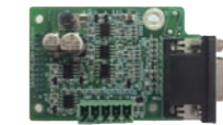
带分频输出sincoS编码器卡(S610用) Frequency divider output sincoS encoder card(For S610)
