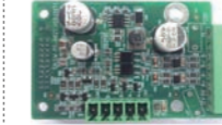
带分频输出ABZ编码器卡(S610用) Frequency divider output ABZ encoder card(For S610)
